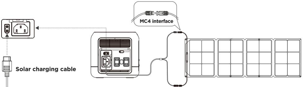
When using EcoFlow solar panels to charge this product, please connect the product according to the specifications in the user manual.
